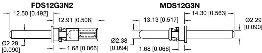
**Material and Finishes:** Precision machined copper alloy with gold flash over nickel. Other finishes are available.
