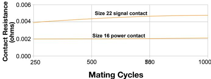
Humidity condition per EIA-364-31B, Method II (condition A) after 250, 500 and 1,000 cycles.
