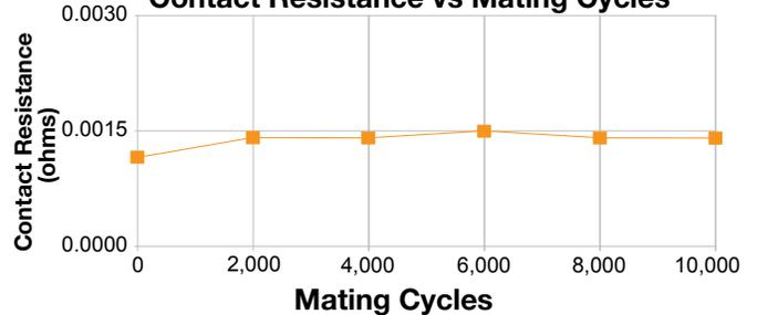
Contact resistance test under 10,000 cycles mechanical operation using GFSH89 with 12 AWG wires and size 16 contacts under load (not utilizing signal contacts).
