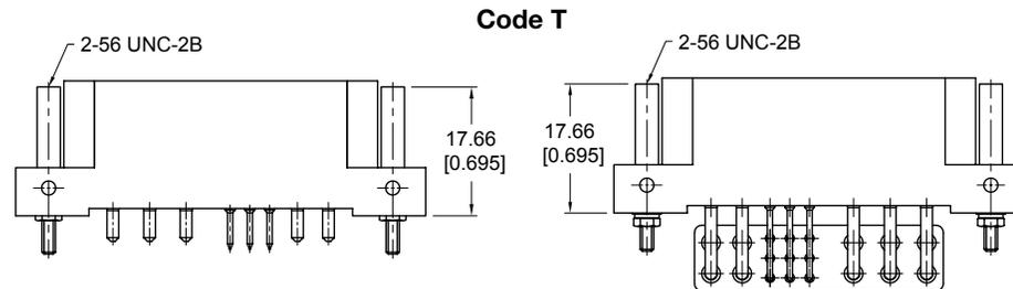
**Note:** For GFSH624, only PCB male fixed jackscrew and Panel female rotating jackscrew is available.
