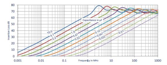
The graph above shows various capacitance values (in  $\mu$ F) and their corresponding Insertion Loss/Filtering Performance For example: a 10 $\mu$ F filter (dark blue, the left-most curve) provides full filtering (60+dB of Loss) by 0.6MHz or 600kHz
